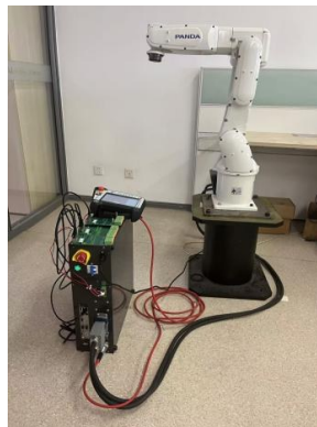
Fig. 8 EtherCAT automatic configuration experimental platform
